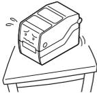
If the surface is not flat and level, this may result in poor print quality. This may also cause malfunction and shorten the life span of the printer.
