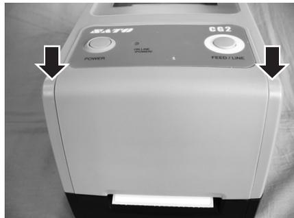
**7** When the printer is offline, the ON LINE (POWER) lamp blinks. Press the FEED/LINE button ①. The printer is online and the ON LINE (POWER) lamp lights. When the printer is ready, press the FEED/LINE button to output the top part of the paper.
