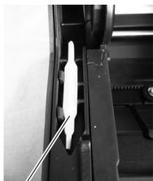
Potentiometer adjustment screwdriver
