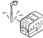
Do not place the printer in a location where it will be splashed with water or oil. Water or oil entering inside the printer may cause a fire, electric shock, or malfunction.
