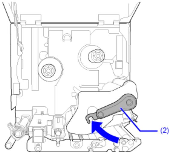
3. Pull the feed lock latch (3) to unlock the feed roller and media sensor assembly.
