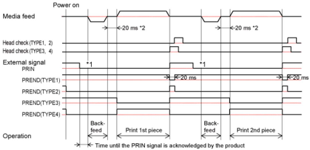
\*1 Keep the PRIN (Print Start) signal until the PREND (Print End) signal is outputted.
