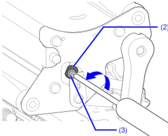
**5. Turn the adjust collar (2) to adjust the head pressure balance.**
