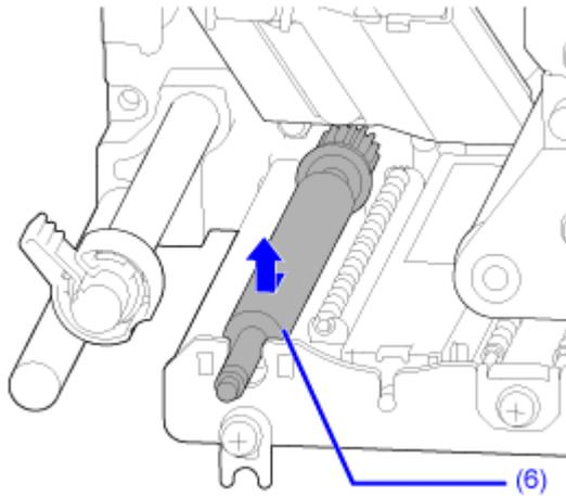
7. Insert the gear end of the new feed roller (6) fully into the center frame of the product.
