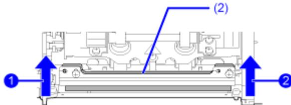
**6. Hold the ribbon adjustment plate (2) in the set position **1** and tighten the two screws **2**.**
