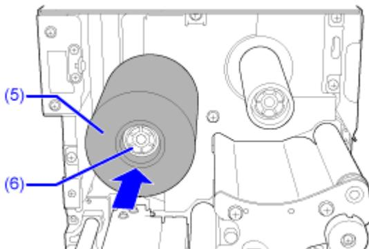
5. From the ribbon supply spindle (6), pass the ribbon below the print head (7) and to the ribbon rewind spindle (4).
