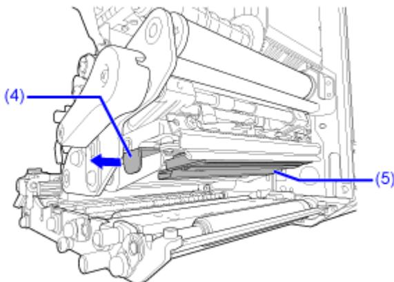
7. Pull out the print head (5) and remove all the connectors (6) from the defective print head (5).
