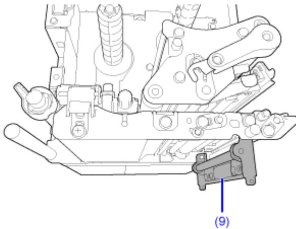
You can remove the pressure plate to clean it easily.
