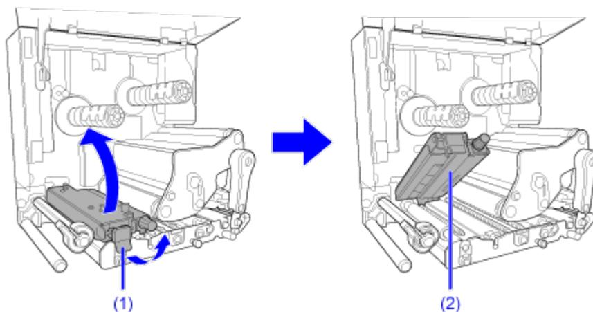
2. Press the feed roller and media sensor assembly (2) down until the feed lock latch (1) is locked.
