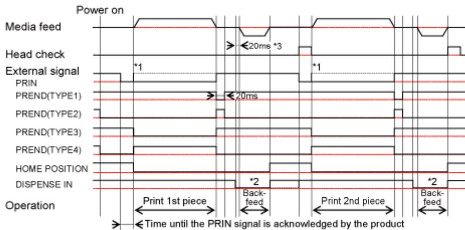
\*1 Keep the PRIN (Print Start) signal until the PREND (Print End) signal is outputted. And then, turn the PRIN (Print Start) signal off before the PREND (Print End) signal detects that printing has ended.
