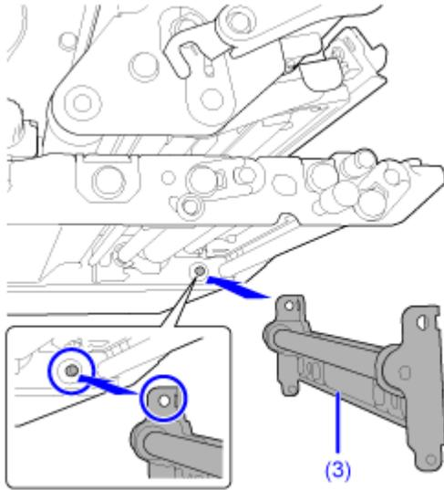
7. Align the position of the screw (4) to the mounting hole on the front side of the pressure plate (3) ①, and tighten them ②.
