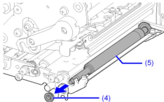
6. Pull out the platen roller (5) from the product and replace it with a new platen roller.
