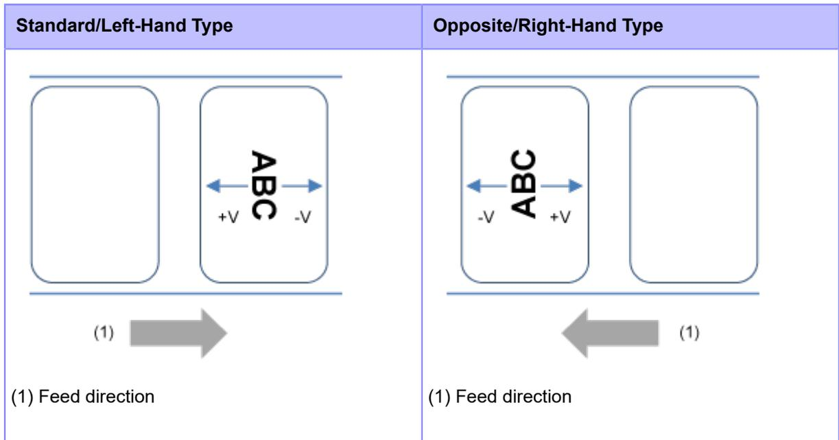
The setting range is from -792 to +792 dots.
