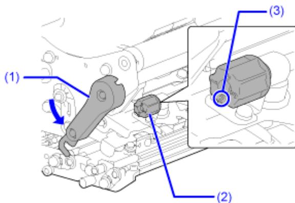
4. **Use the slotted screw driver to turn the adjustment dial (2), and then set the pressure balance according to the media width and media thickness.**
