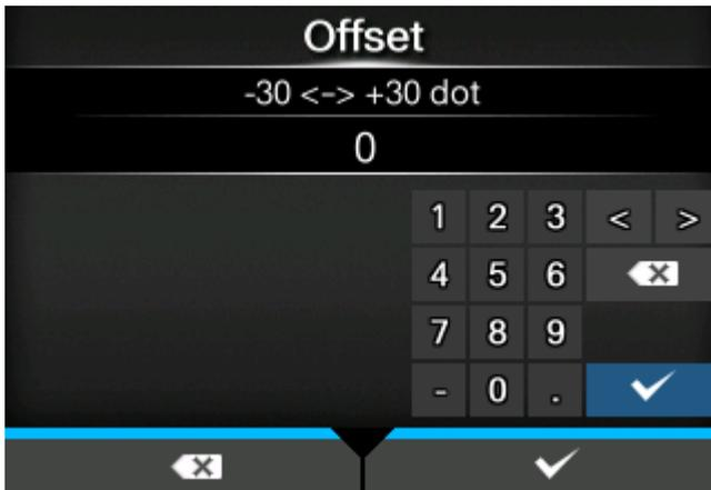
5. Change the setting value. Press the ◀/▶/▲/▼ buttons to select a number and then press the ← button to enter the number to the text box.
