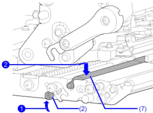
9. Place the bearing (6) back to the chassis and the shaft of the pressure roller (7).
