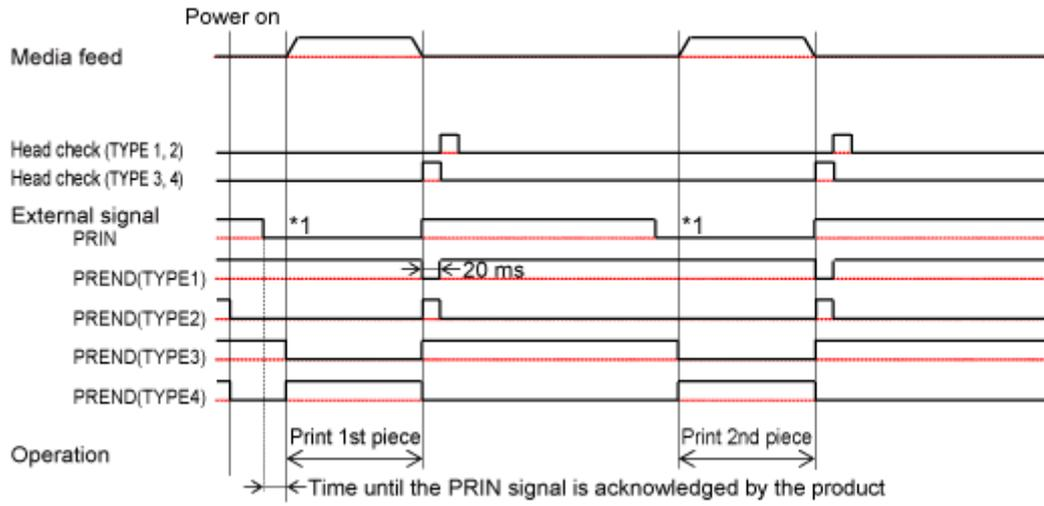
\*1 Keep the PRIN (Print Start) signal until the PREND (Print End) signal is outputted.
