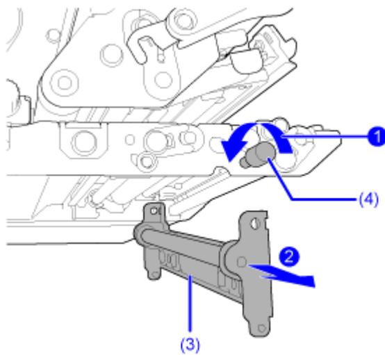
6. Insert the protrusion of the product's center frame securely into the mounting hole on the leading-edge side of the pressure plate (3).
