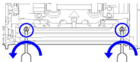
**5. Adjust the ribbon adjustment plate (2) as shown below.**
