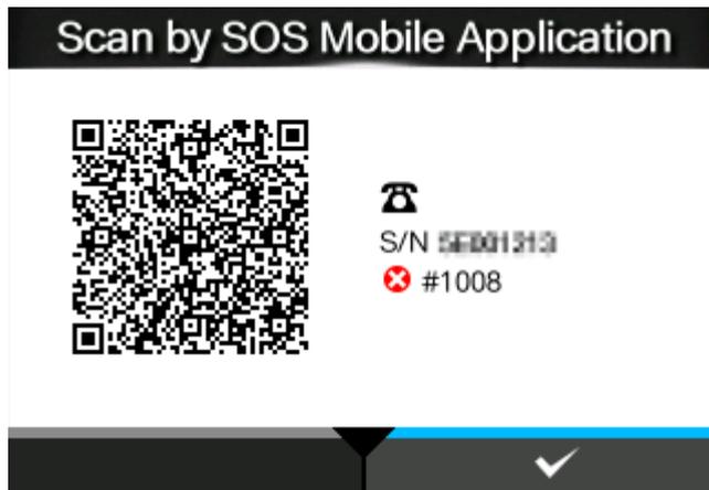
Scan the QR code with the specialized SOS application from a tablet device or smartphone. After scanning the QR code, the menu for the specialized SOS application appears.
