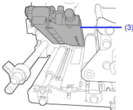
You can remove the media sensor cover to clean the surface easily.
