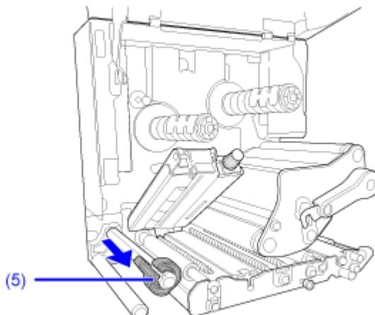
5. Pass the media between the media shaft (6), below the feed roller and media sensor assembly (4), and the print head assembly (7) and extend it out the discharge outlet (8).
