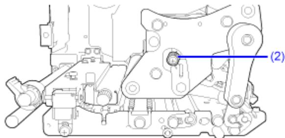
**4. Loosen the screw (3) attached to the adjust collar (2).**
