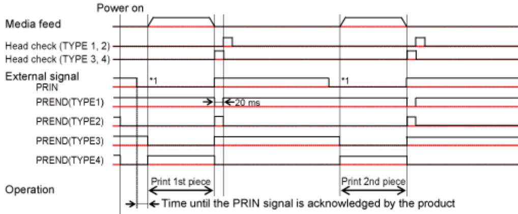
\*1 Keep the PRIN (Print Start) signal until the PREND (Print End) signal is outputted.
