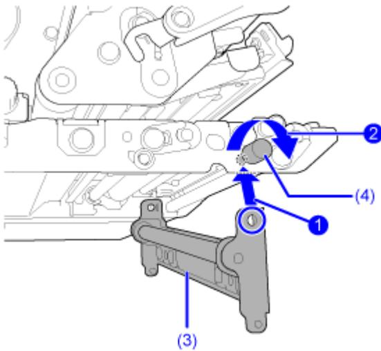
8. Push the center of the pressure plate (3) to latch it in place.
