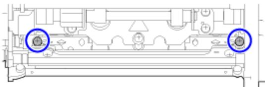
**4. Loosen the two screws using the Phillips screwdriver.**
