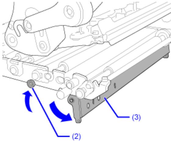
5. While supporting the pressure plate (3), loosen screw (4) until the front of the plate falls **1**, and then pull the pressure plate (3) forward to remove it **2**. Then, replace it with a new pressure plate.
