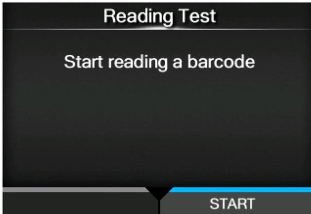
If reading is successful, the barcode type and data read are displayed on the screen. Only the first 23 bytes of data are displayed.
