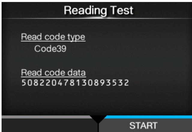
If reading is unsuccessful, or the displayed results of the read are not correct, adjust the position of the barcode checker. For details on how to use the barcode checker, refer to the manual that came with the barcode checker.
