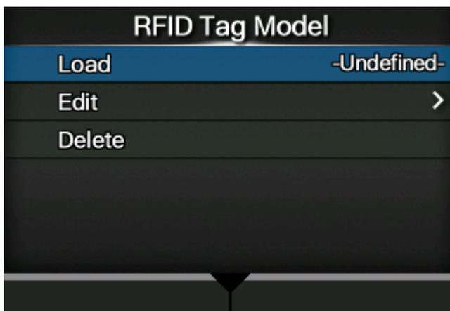
6. Press the ▲ / ▼ buttons to select the RFID tag model to load.
