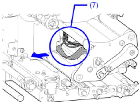
**10. Install the print head (5) to the print head assembly.**
