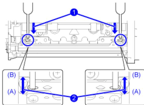
**6. Tighten the two screws.**
