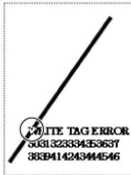
When using a small-size label (about the size of P30 X W40 mm (P1.18" X W1.57"), for example) or not enough for setting margin, the slash and error message are printed overlap on each other. The overlapped area are inverse from black to white. There is no dump printing.
