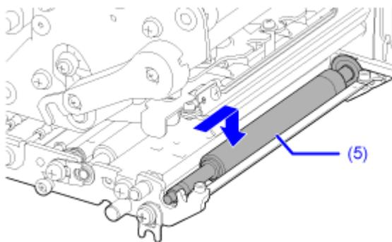
8. Place the bearing (4) back to the chassis and the shaft of the platen roller (5).
