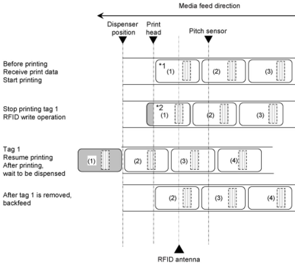
\*1 Because the EPC code read, RFID read [DC2]PJ, UID/EPC/IDm print <TU>, and UID/EPC/IDm return <RU> commands acquire the information at this inlay position, do not use them if the Tag Offset is set to other than an initial value.
