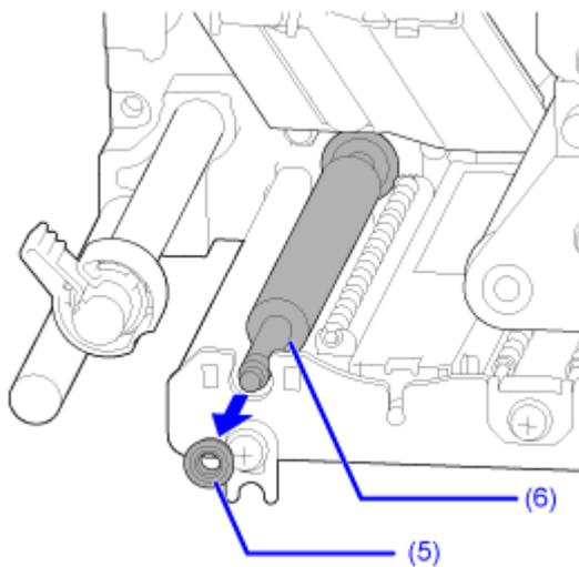
6. Pull out the feed roller (6) from the product and replace it with a new feed roller.
