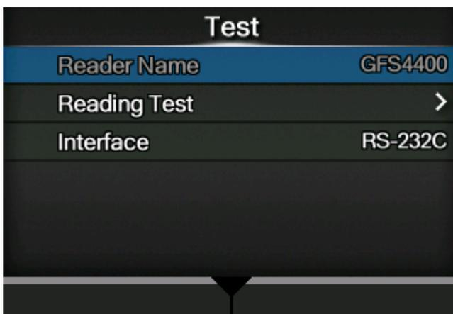
7. Press the ▲/▼ buttons to select [Reading Test], and then press the ⬅ button.
