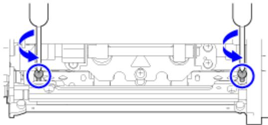
**5. Insert the slotted screwdriver into the regulation apertures ① on the left and right sides. Adjust the head position by turning the slotted screwdriver in the relevant direction ②.**
