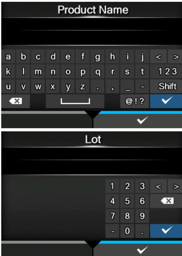
12. If the format contains a counter, enter the start value of the counter with the on-screen keyboard or a USB scanner, keyboard or keypad.
