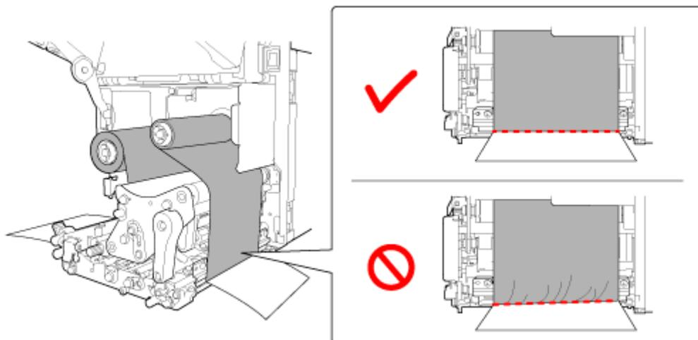
**8. Repeat the procedure from steps 1 through 6 until the ribbon tension is even on both sides.**
