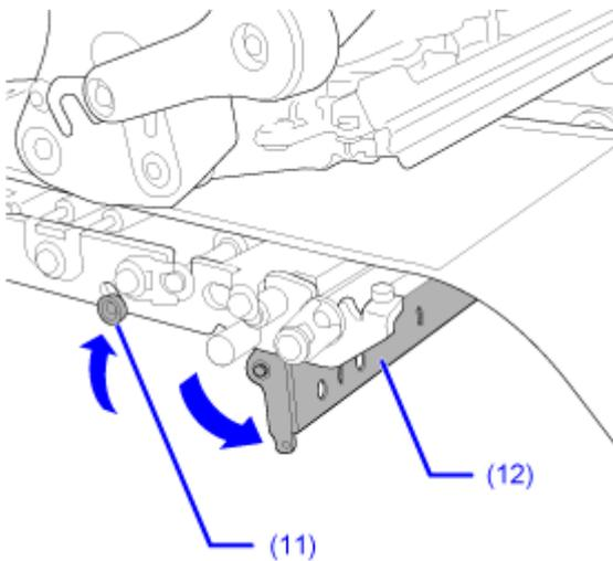
9. Pass the liner (10) through the gap of the pressure plate (12).
