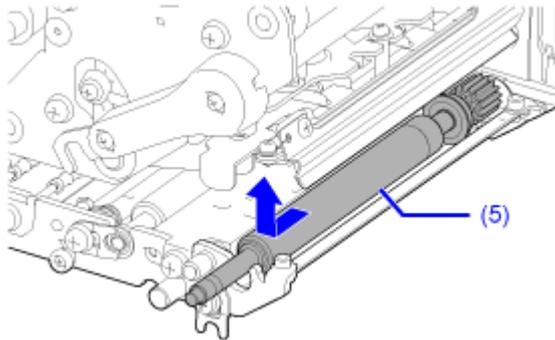
7. Insert the gear end of the platen roller (5) fully into the center frame of the product.
