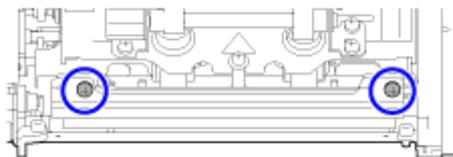
4. Loosen the two screws attached to the ribbon adjustment plate.
