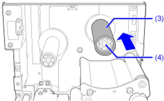
If there is any ribbon on the ribbon rewind spindle, remove it from the spindle before installing new ribbon.
