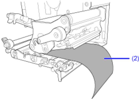
6. Turn the head lock lever (1) counterclockwise to lock the print head.
