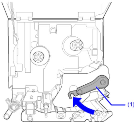
3. **To expose the adjustment dial (2) beside the head lock lever as shown, turn the head lock lever (1) back until before it locks.**
