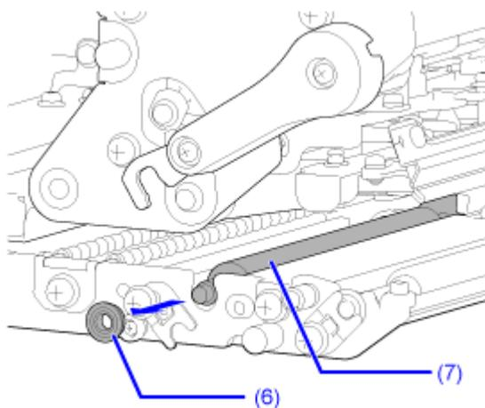
7. While pushing the tab (2) up ①, pull out the pressure roller (7) from the product ② and replace it with a new pressure roller.
