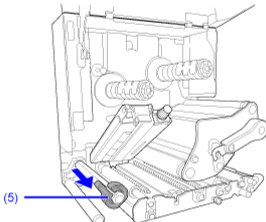
5. Pass the media between the media shaft (6), below the feed roller and media sensor assembly (4), and the print head assembly (7) and extend it out the discharge outlet (8).
