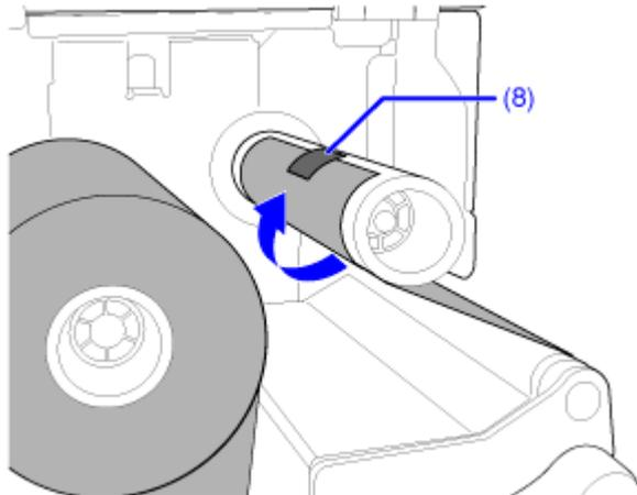
9. Turn the ribbon rewind spindle (3) clockwise for several rounds to wind the ribbon while removing the slack from the ribbon.
