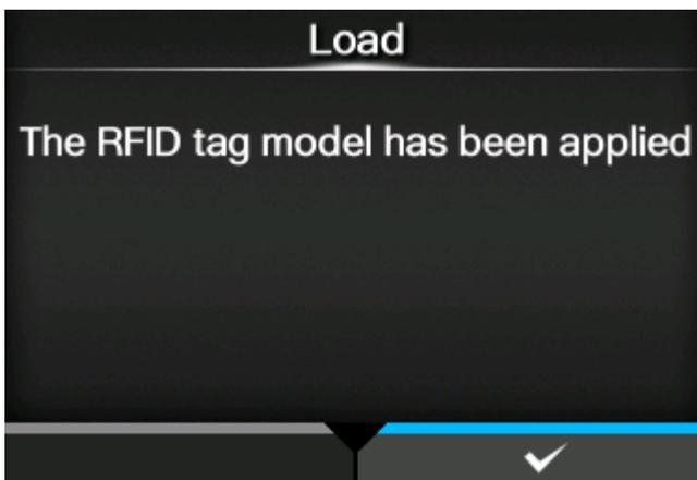
The settings loaded from the RFID tag model are applied to the product. The name of the loaded RFID tag model appears on the right side of [Load] on the [RFID Tag Model] menu.
