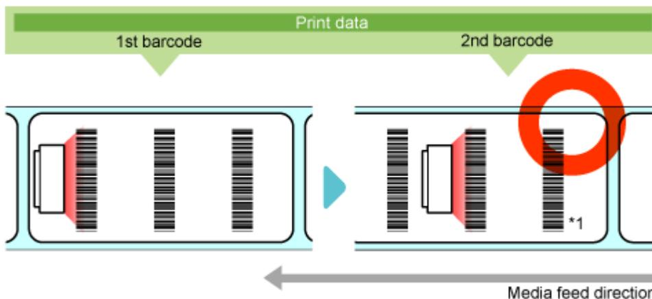
\*1 Even if the number of barcodes the barcode checker reads exceeds the number of barcodes in the print data, it is considered to be successful.
