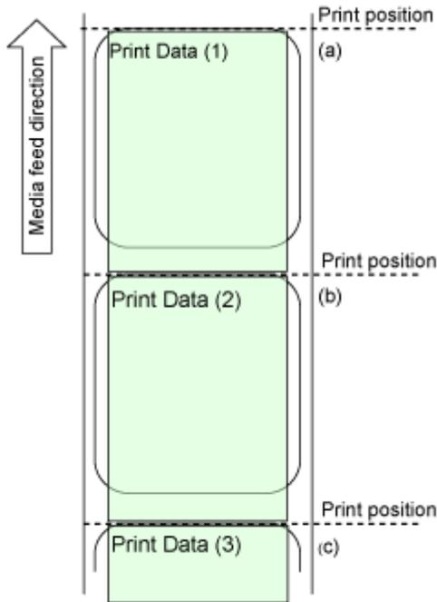
Print data (1) stops printing at print position (b). The next printing is done from print position (b).
