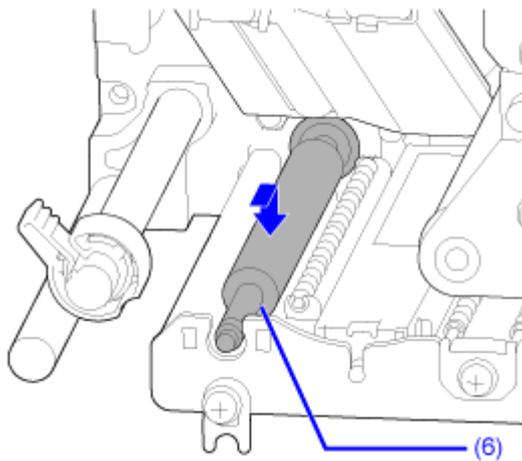
8. Place the bearing (5) back to the chassis and the shaft of the feed roller (6).
