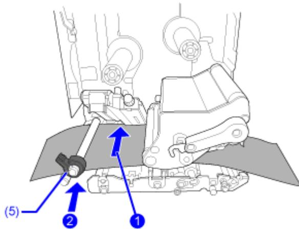
7. Turn the head lock lever (2) counterclockwise to lock the print head (1), and then press the feed roller and media sensor assembly (4) down until the feed lock latch (3) is locked (2).
