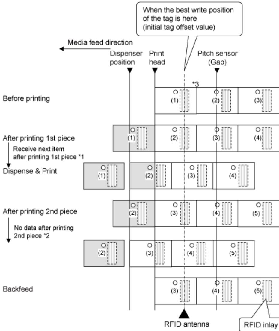
\*1 If the next data is received after printing finishes, then the next print operation is done and dispensing stops at the dispensing position.
