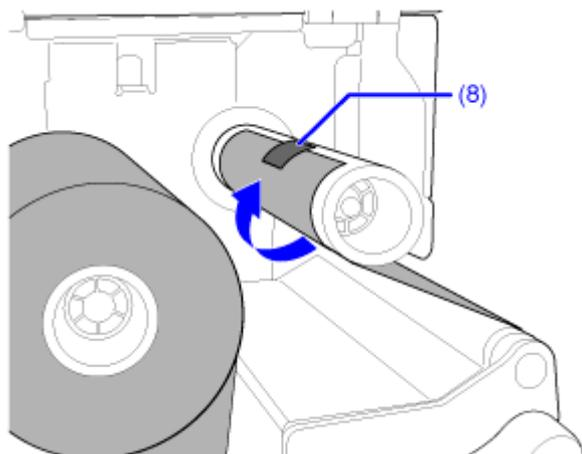
7. Turn the ribbon rewind spindle (4) clockwise for several rounds to wind the ribbon while removing the slack from the ribbon.
