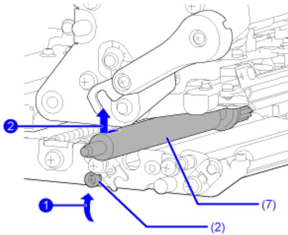
8. While pushing the tab (2) up ①, insert the gear end of the pressure roller (7) fully into the center frame of the product ②.
