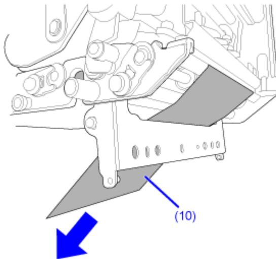
**12. Push the center of the pressure plate (12) to latch it in place.**
