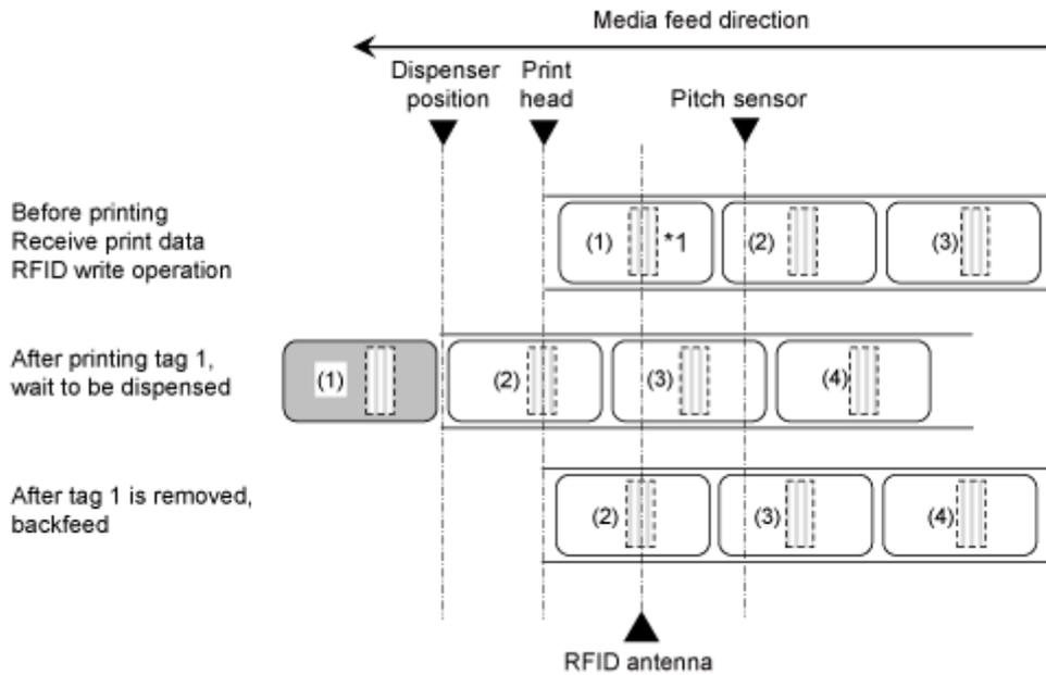
\*1 The EPC code write <IP0> command writes the data at this inlay position. The EPC code read, RFID read [DC2]PJ, UID/EPC/IDm print <TU>, and UID/EPC/IDm return <RU> commands acquire the information at this inlay position.
