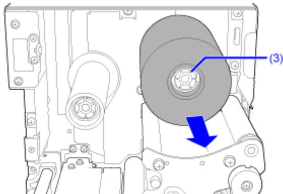
**4. Pull to remove the empty core from the ribbon supply spindle (4).**
