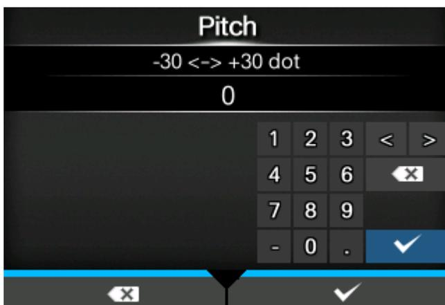
5. Change the setting value. Press the ◀/▶/▲/▼ buttons to select a number and then press the ← button to enter the number to the text box.
