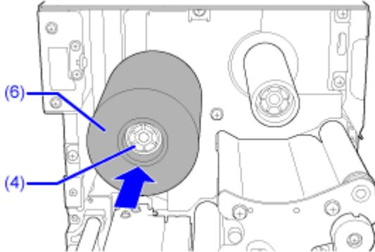
**7. From the ribbon supply spindle (4), pass the ribbon below the print head (7) and to the ribbon rewind spindle (3).**
