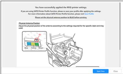
For CL4NX Plus, CL6NX Plus, CL4NX-J Plus, CL6NX-J Plus, CT4-LX and S84NX, click [Reboot Printer] button so that the printer can automatically adjust the position of the antenna to suit the RFID tag.
